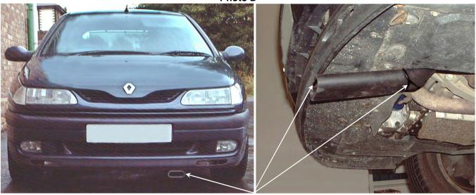
Taking all of the necessary safety precautions as per the manufacturers instructions, raise the front of the vehicle. Drill / pierce two 3mm holes in the front lower spoiler trim and the lower cross member, secure the rubber cold air scoop to the spoiler trim / cross member using the 2 long plastic ties supplied. Insert the flexi cold air hose into the top of the scoop. (It may be necessary to cut a section out of the air deflector flap to ensure a good fit for the scoop).
