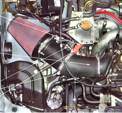
**4.** Insert the hose from the rochester valve into the hole in the side of the new intake hose.
