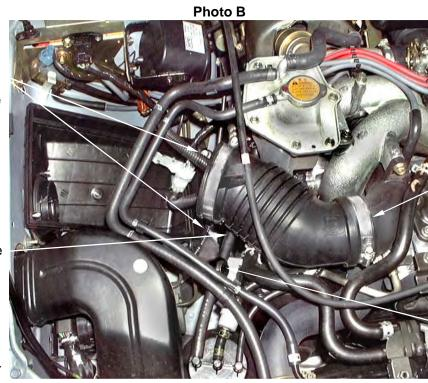
3. Unclip and remove the intake hose from the plastic intake pipe.
