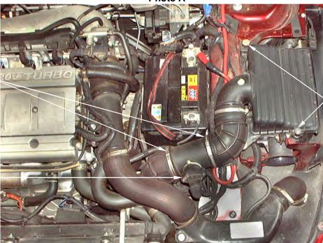
**3.** Unscrew and remove the complete air box assembly.
