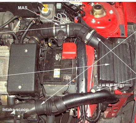
**3.** Remove the rubber intake hose from the plastic intake scoop.
