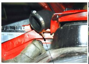
**1.** Fit the new intake hose to the MAS and secure with a hose clip bracket using the supplied. Do not fully tighten the clip yet.
