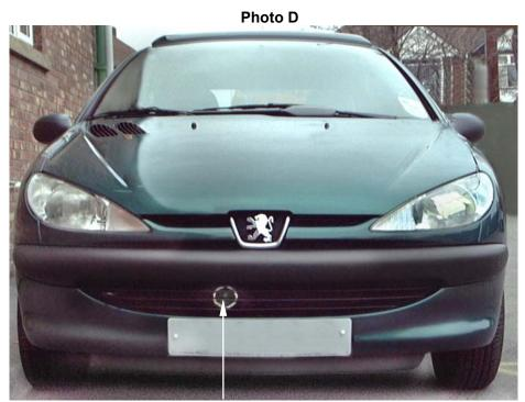
Pierce / drill a 3mm hole in the end of the flexi cold air hose, feed the hose down to the front lower grille and secure it to the grille using a plastic tie supplied.
