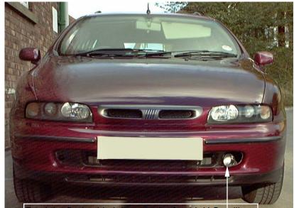
Feed the flexi cold air hose to the front L.H.S. grille and secure in place using a long plastic tie supplied.
