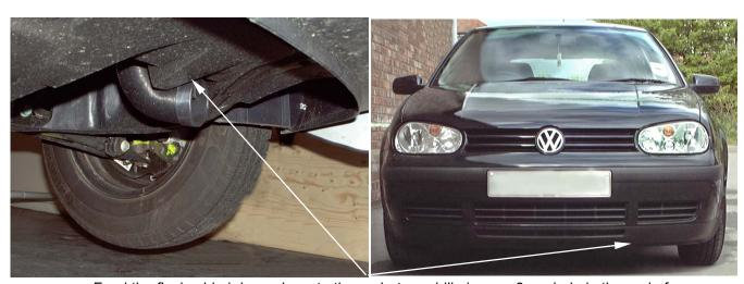
Feed the flexi cold air hose down to the undertray, drill pierce a 3mm hole in the end of the flexi cold air hose and undertray panel and secure with a long plastic tie supplied.
