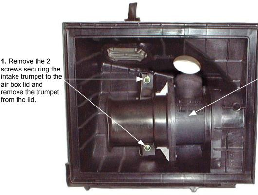
2. Slide the MAS out of the air box lid and remove the seal.
