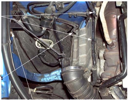
3. Attach the new mounting bracket to the original air box mounting point using the original mounting screw.
