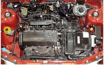
1. Release the hose clip securing the intake hose to the throttle body.
