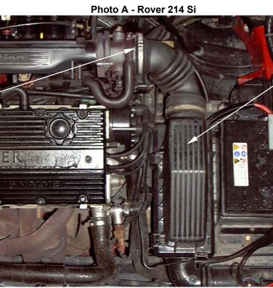
2. Unclip the airbox lid from the airbox assembly and remove the intake hose, air box lid and air filter from the vehicle.
