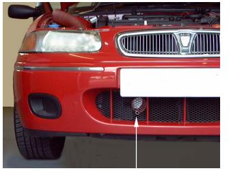
Remove the plastic trim next to the radiator. Pierce a 3mm hole in the end of the cold air hose and then secure the hose to the lower grille with a plastic tie provided.
