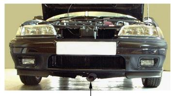
Feed the flexi cold air hose down to the centre of the front lower spoiler. Pierce a 3mm hole in the bottom of the cold air hose and attach the hose to the front towing eye using the plastic tie provided. Ovalise the end of the cold air hose to increase ground clearance.
