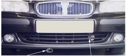
If the car has air conditioning fitted it may be necessary to feed the cold air hose down to the front lower spoiler. The hose should be ovalised to obtain sufficient ground clearance and then secured in place by drilling / piercing a 3mm hole in the end of the hose and spoiler and attaching them together with the medium plastic tie supplied.
