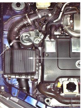
2. Unclip and remove the air box lid and filter element from the base. Leave the air box base in place.
