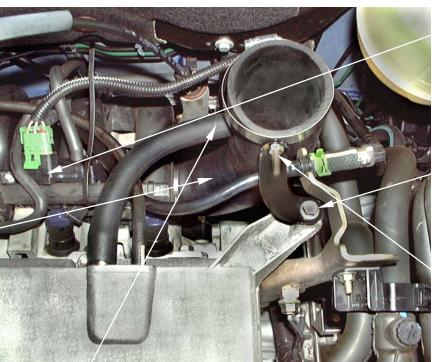
3. Attach the new breather hose onto the cam cover breather and secure using a small hose clip. Insert the breather hose into the hole located in the side of the intake hose.
