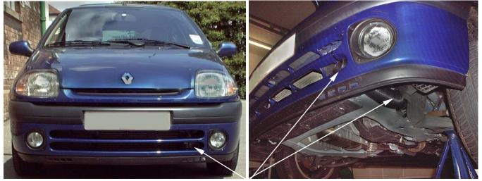
itions as per the manufacturers instructions carefully raise r hose past the side of the arch liner and feed towards the and remove a plastic cover from the side of the radiator e into the front grille area, pierce a 3mm hole in the end of the grille using a plastic tie supplied.
