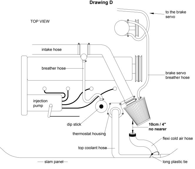
Lengthen the flexi cold air hose to 51cm / 20". Feed the cold air hose down between the gearbox and radiator to the front lower bumper. Use a long plastic tie to attach the top of the cold air to the coolant hose
