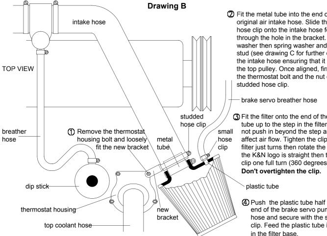
2 Fit the metal tube into the end of the original air intake hose. Slide the studded hose clip onto the intake hose feed the stud through the hole in the bracket. Fit the flat washer then spring washer and nut to the stud (see drawing C for further detail). Align the intake hose ensuring that it is clear of the top pulley. Once aligned, firmly tighten the thermostat bolt and the nut on the
