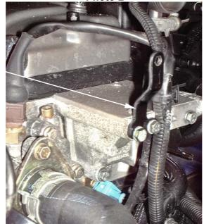
**1.** Attach the new mounting bracket to the original mounting point using the original screws.
