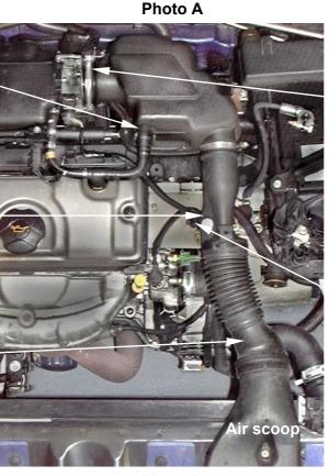
**4.** Loosen the hose clip and remove the air box assembly.
