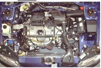
**1.** Unclip and remove the breather hose from the side of the air box.
