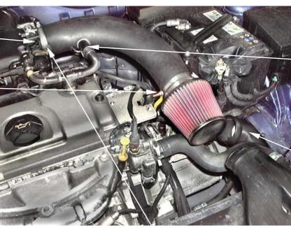
**4.** Fit the filter assembly to the new intake hose. Rotate the filter until the K&N logo is straight then tighten the studded clip.
