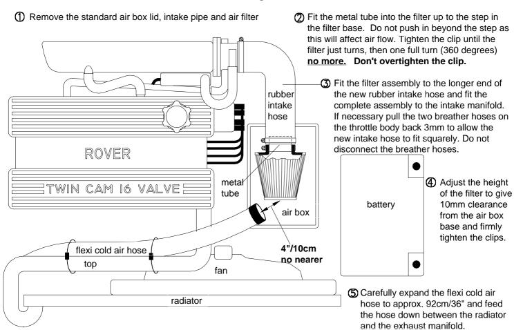
**6** Position the hose to finish approx. 10cm/4" from the filter **no nearer** and tie the flexi cold air hose to the radiator top hose with the two long plastic ties supplied.
