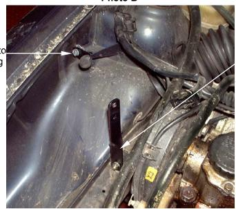
2. Attach the rubber bobbin and bracket to the rear air box mounting point using the nut and washers supplied.
