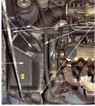
**4.** Release the 3 nuts securing the air box base to the inner wing. Lift out the air box base from the mountings and remove from the vehicle.
