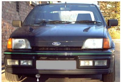
Feed the flexi cold air hose to the front lower spoiler and tie the hose to the metal cross member using one of the plastic ties. It may be advisable to ovalise the end of the hose to increase ground clearance.
