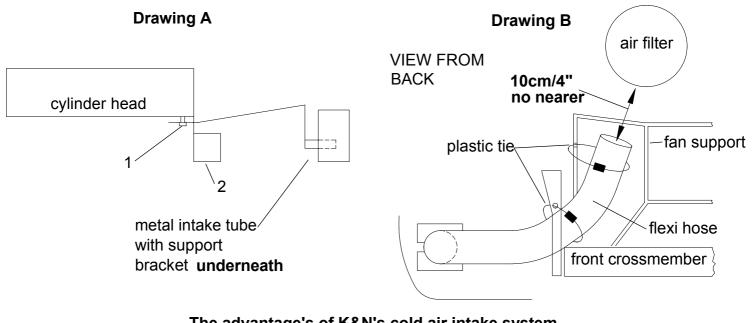
The advantage's of K&N's cold air intake system Cooler air being denser, will show positive improvement in power over filter systems that draw hot air from the engine bay.
